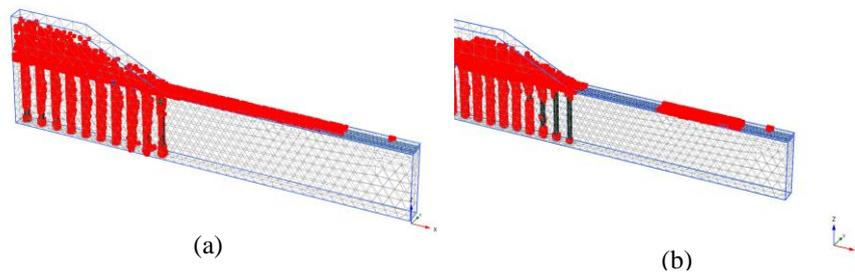
**Fig. 6.** Formation of plastic points for  $L_{ESC} = 10$  m after (a) construction and (b) consolidation period is over
