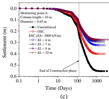
**Fig. 3.** Settlement variation of incorporating the impact of (a) stiffness of encasement, (b) ESC length, and (c) length of encasement
