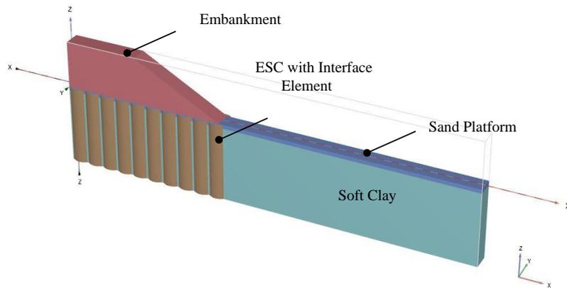
**Fig. 1.** Numerical model of the embankment with full-length ESC.
