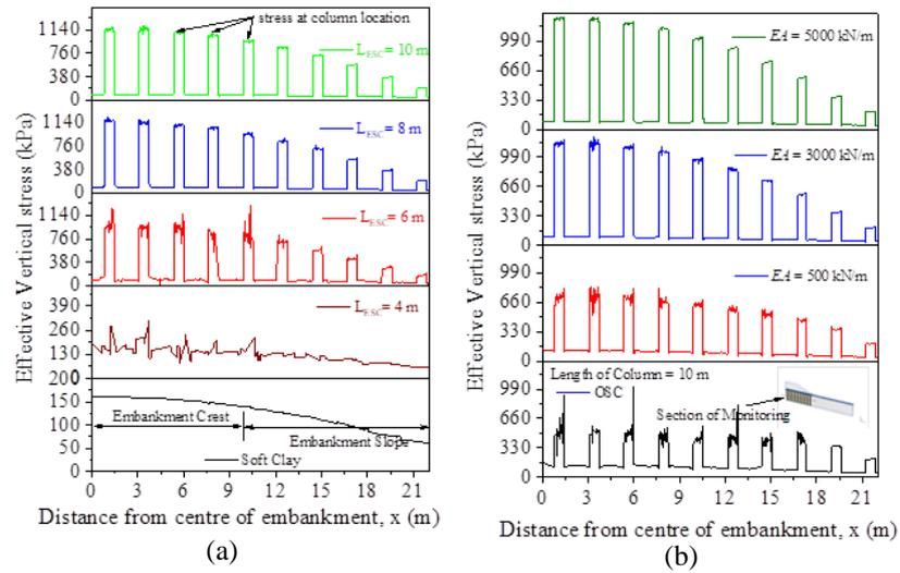
**Fig. 4.** Impact of (a) ESC length and (b) stiffness of encasement on vertical stresses
