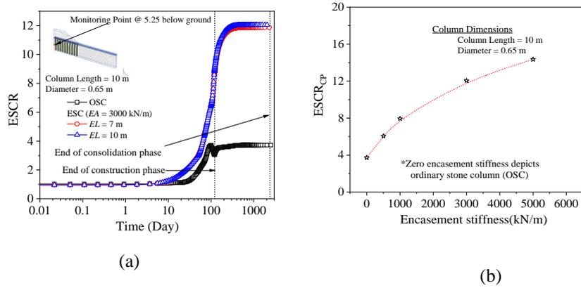
**Fig. 5.** Impact of (a) ESC length and (b) stiffness of encasement on the ESCR
