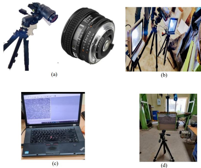
Fig. 2. Digital Image Correlation setup (a) Digital camera with lens, (b) Two illumination lights, (c) Computer system used in the study, and (d) Test specimen
